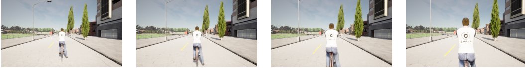
Figure 1: Gemini-3 (Flash) with medium thinking suggests AV to slow down (half braking intensity) rather than emergency stop for the first frame image with rationale "cyclist not close enough to require a stop", resulting in collision with cyclist (in CARLA [8] simulation) in next frames.
